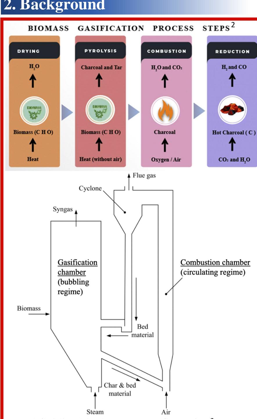
Dual fluidized bed reactor configuration<sup>3</sup>:
